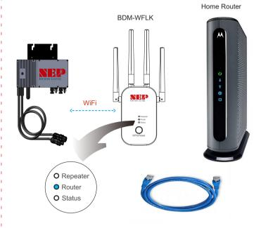
BDM-WiFi devices are pre-configured to link to BDM-WFLK. BDM-WFLK links to home router through Ethernet cable.
