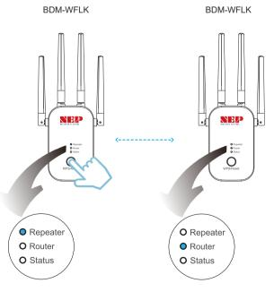
Hold "WPS/Reset" for 6 second, (1st LED light flashes 6 times) and release, BDM-WFLK switches between two modes.
