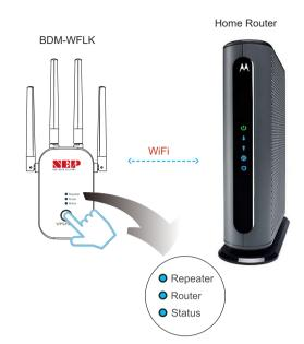
Press "WPS/Reset" for 2 second and release, three LED lights start flashing BDM-WFLK enters WPS mode.
