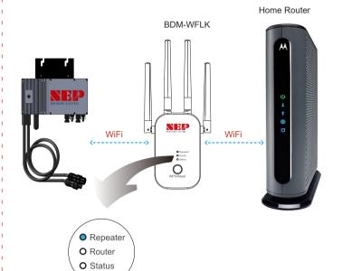
BDM-WiFi devices are pre-configured to link to BDM-WFLK. BDM-WFLK communicates with home router through WiFi (WiFi configuration is required).
