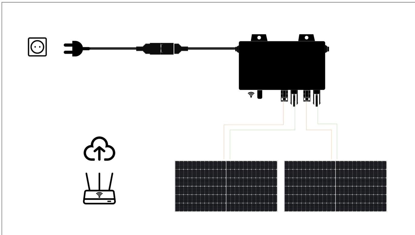
For balcony solution, there is only one inverter in the system. The monitoring is realized by WIFI connection between WiFi dongle on the inverter and home router.
